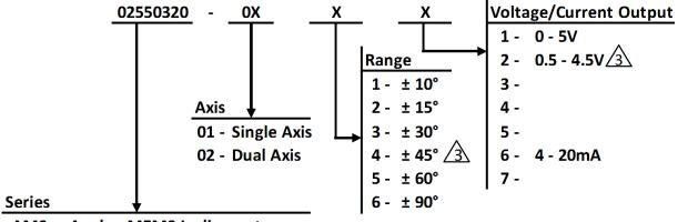
AMS - Analog MEMS Inclinometer (Resolution: 0.01° & Zero Temp Drift: ±0.006°)
