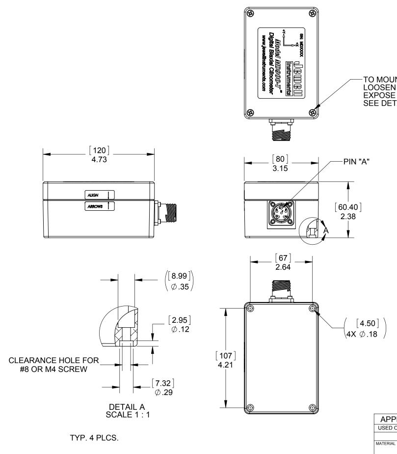
TO MOUNT UNIT: LOOSEN FOUR (4) SCREWS, REMOVE COVER TO EXPOSE FOUR MOUNTING HOLES SEE DETAIL A
