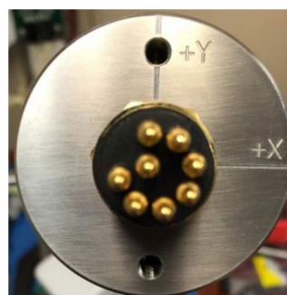
Figure 2: Male Bulkhead Connector showing +X & +Y axis Orientation (left) and Pin Number Orientation (right)
